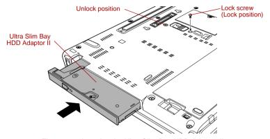
Figure 4-20 Inserting the Ultra Slim Bay HDD Adaptor II
